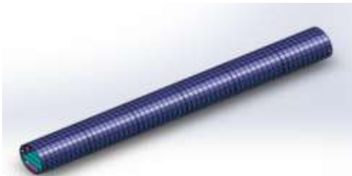
Fig.10 Assembly of complete fuselage of length 36m
